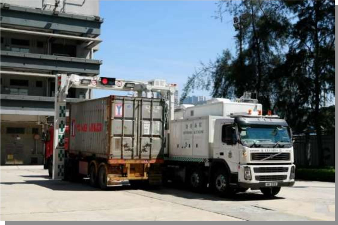
A Mobile X-ray Vehicle Scanning System scanned a container truck at Kwai Chung Customhouse, Hong Kong
