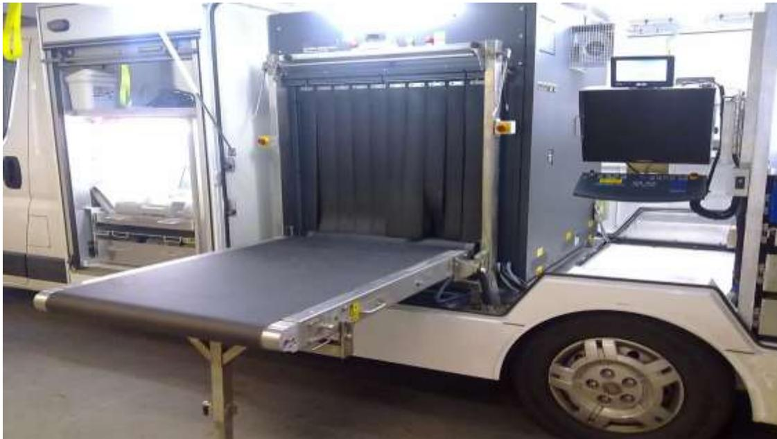
**Interior of the Mobile X-ray with conveyor deployed**
