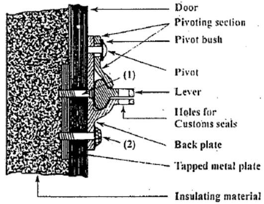
(1) Set-screw head completely deformed by welding. Not accessible when door sealed
