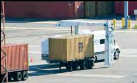
**Truck being screened by a mobile HCV system**
