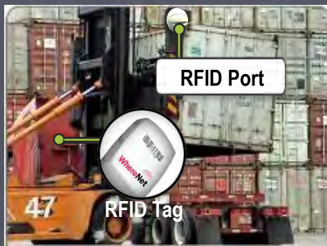
RFID tag on top-pick forces the truck or chassis tag to transmit its ID. ID is auto transferred back to the top-pick
