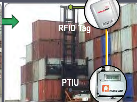
Container and Top-pick are automatically associated based on PTIU sensor and location
